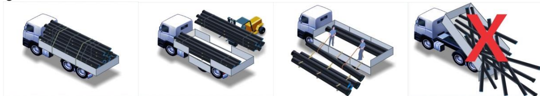
Figure 44 - Transport and unloading precautions
