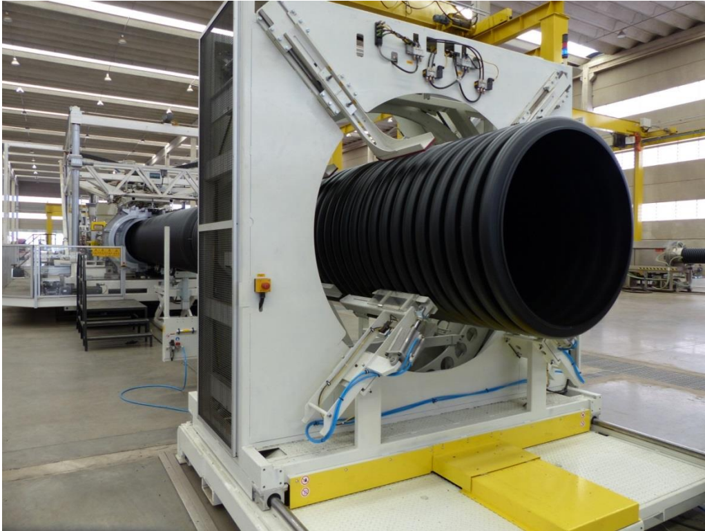
Figure 1 - KNTS Drain Pipe Manufacture
